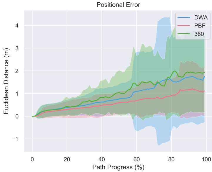
Figure 20: This figure shows the evolution of the Euclidean distance error (in meters) between the estimated and actual positions across 75 simulation experiments (25 in the restaurant-world (see Figure 16) and 50 in the station-world (see Figure 17)). In some cases, large positional errors caused runs to last indefinitely. Whenever an algorithm exceeded three minutes, the test was aborted and labeled as a failure. These aborted runs were excluded from the plots.
