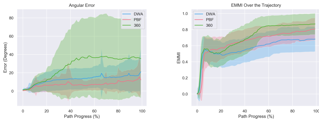
Figure 23: The left graph shows how the error in orientation error, measured in degrees (based on Euler angles), evolves between the estimated and actual orientations in the experiments conducted at the ISR Testbed. The figure on the right illustrates the evolution of the EMMI value. Initial zero values can be disregarded, as the entropy calculation had not yet commenced. Data of tests which did not reach the goal successfully were excluded.
